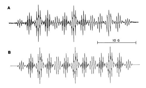
Figure 1. A: ESR spectrum of phenoxazine- $\underline{N}$ -oxyl in benzene at room temperature.
